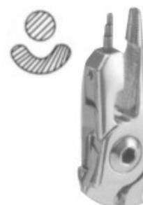
709-497-130 Tweed Loop Forming Plier 13 cm, 5" convex/concave beak makes precise omega loops. Ti has 3 forming sections: .045", .060". And .075". Etched tip surfaces prevent wire slippage.
