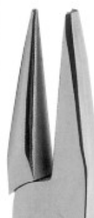
709-192-130 Optical Plier For Loops 13 cm, 5" This durable plier has fine tips for making precision bends and adjustments, and gives you easy access to hard-to-reach intraoral areas. The upper jaw is rounded, fitting into a concave groove in the lower. Use wires up to .028".
