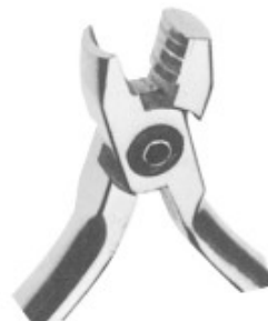
709-395-130 De La Rosa Arch Forming Plier 13 cm, 5" grooved. Designed to form and contour arch wires with or without torquing on round or rectangular wire. The beak has grooves of 0.41mm, 0.46mm, 0.56mm
