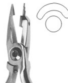
709-383-130 Omega Loop Forming Plier. 13 cm, 5" For making perfect omega loops in square or rectangular wires up to 0.56x0.71mm.
