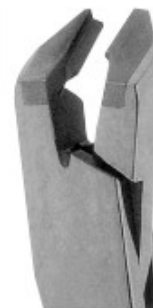
709-183-130 Intraoral Detailing Plier 13 cm, 5" Fabricate delicate offsets in archwire – accurately, quickly. Ideal for bends to engage lingually positioned teeth. Also good for by-pass and 2nd order bends. Makes 1mm bends.
