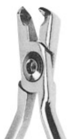
709-326-130 Distal End Cutter (non-holding). 13 cm, 5" A precision cutter designed for distal arch cutting. Cutting angle of 72 degree allows cutting of wire very close to distal end of buccal tube. Caution: maximum cutting capacity arch wire up to 0.56x0.71 mm rectangular, round wires up to 0.51 mm.
