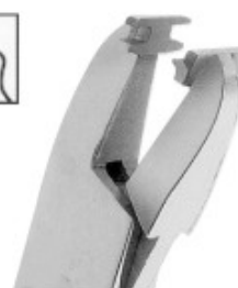
709-174-130 Intraoral "V" Notch Stop Plier 13 cm, 5" Now make precise 1mm "V" stops right in the mouth. Prevents wires from disengaging from the buccal tubes. Notches up to .018" round and .016" x .022" rectangular.
